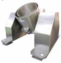
• **Hydroextraction:** When the feeding step is completed, the basket speed is increased to a preset value. • **Product discharge:** Once basket rotation has stopped, the casing assembly and basket overturn 180° such that
