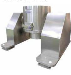
• Product discharge: Once basket rotation has stopped, the casing assembly and basket overturn 180° such that the product is discharged by gravity. The assembly returns to the vertical position and a new cycle can begin. The RC60RIAL can also be used for semi-automatic service: The operator triggers the overturning and the product is recovered in a bin, which eliminates the need for manually removing the product.
